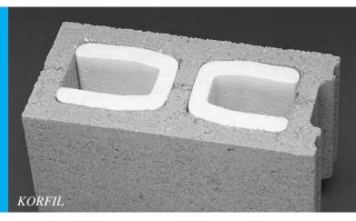
Composition and Materials: KORFIL Inserts are individually molded from expandable polystyrene in a minimum density of 1.3 lbs. per cu. ft. Inserts are packaged at the point of manufacture in heat-sealed, clear polyethylene bags.
