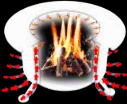
Smoke-Less Fire Systems work through a double-wall, secondary combustion design. When the fire is burning, the walls heat up and the hot air rises through the gap between the two walls. The air then exits the wall cavity through the line of holes around the rim. Pressurized, heated oxygen mixes with the smoke and causes it to reburn.
