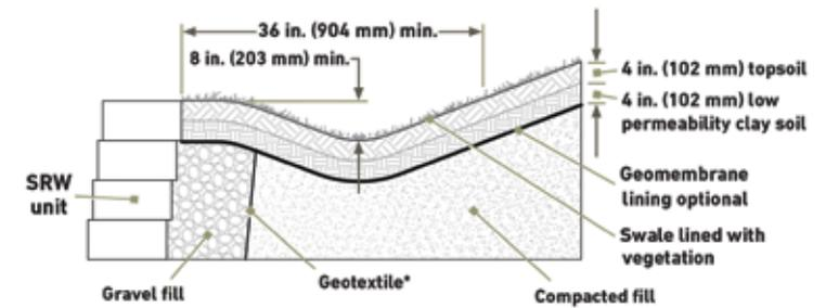
\*Geotextile may be necessary when the infill soil includes fine-grained sand that have the potential to infiltrate the gravel fill
