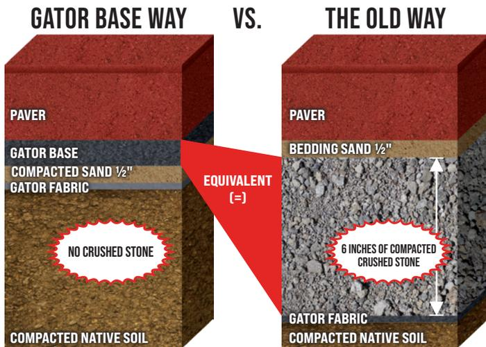
**GATOR BASE REPLACES 6" OF COMPACTED CRUSHED STONE!**
