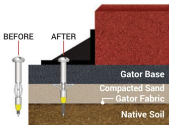
Gator Screws are used to fasten Gator Tile, Mini, Flex or Rigid edge to the Gator Base
