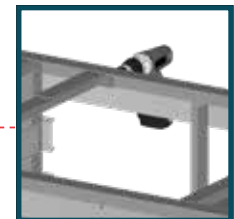
Braces are attached via tab and a self-tapping screw (ST02)
